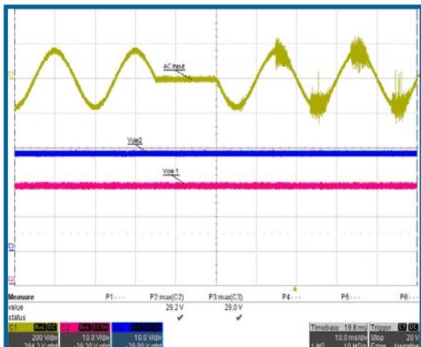
**Input power brake at 230Vac 100% Load - PST21C-28150-28150**
