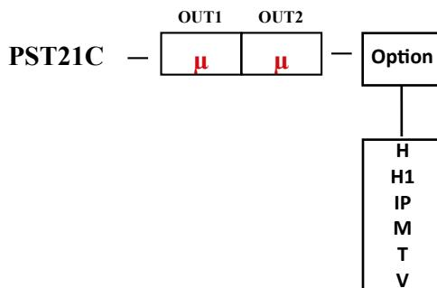
**μ-μ** : Microboard out1, out2 : Up to 2 outputs with micromodules from 2V to 48Vdc 150W (see table page 3)
