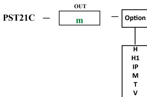
**m** : Miniboard out1 : Up to 1 output with minimodules from 2V to 48Vdc 300W (see table page 3)
