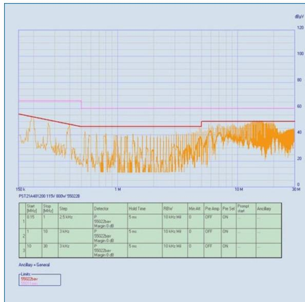
According to EN55022A/B for PST21A-48600-48600 at 230Vac IN/1200W
