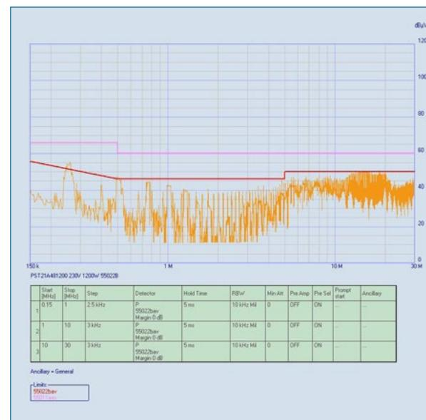
According to MIL-STD461E CE102 PST21A-48600-48600-M at 220Vac IN/800W
