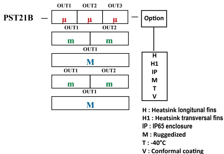
**μ-μ-μ** : Microboard out1, out2, out3 : Up to 3 outputs with micro-modules from 2V to 48Vdc 150W (see table page 1)
